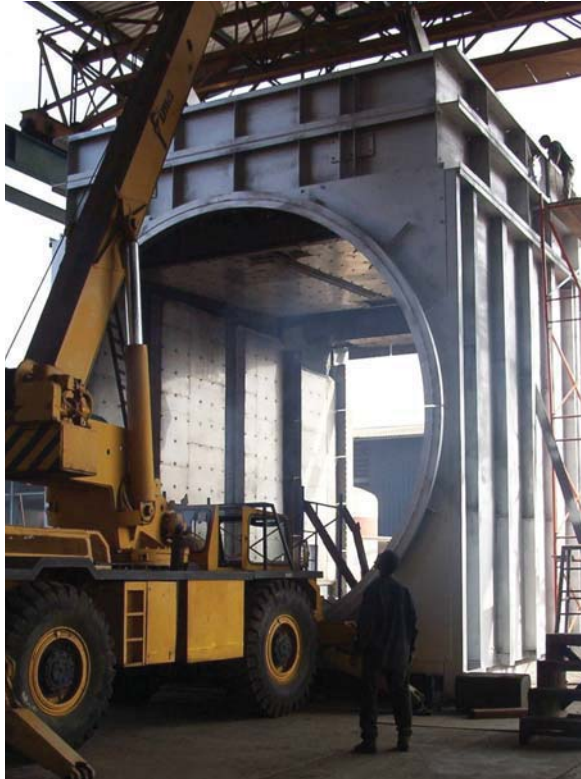
Diverter for a Siemens SGT6 - 4000F GT in Peru
