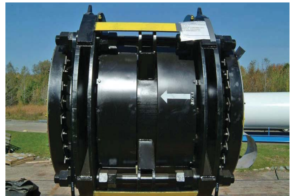
914 mm (36") diameter Universal Metal Expansion Joint for a cycle gas service. Inco 600 redundant ply testable bellows with root rings. 422 psig at 150°C (302°F)
