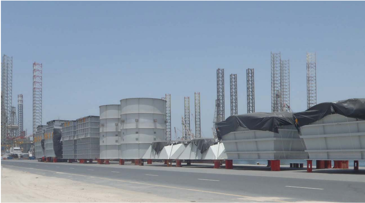
Bypass system for a GE 9E gas turbine in Argentina
