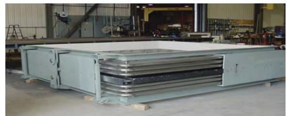
3048 mm (120") square Hinged Refractory-lined Universal Expansion Joint for a refinery. Inco 600 bellows with rounded corners. 2 psig at 650°C (1200°F)
